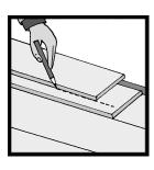
When cutting the last row of boards ensure a 10 mm expansion gap is left. A pull bar will be needed to tap the boards into position. When complete, remove any spacers, cut any PE foil flush with the top of the boards and fit skirting
